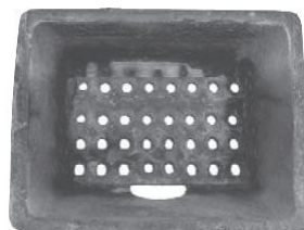
Example of clean grate
