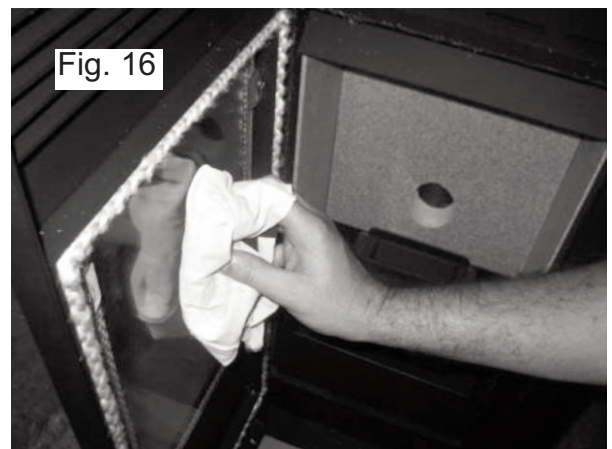
Fig.15 & 16 – Correct cleaning of the glass.
