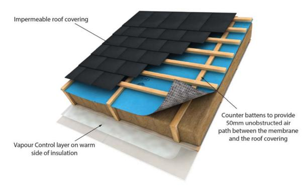
Figure 2: Warm Roof detail with impermeable roof covering
