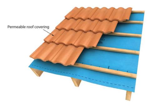
Figure 1: Cold Roof detail with permeable roof covering
