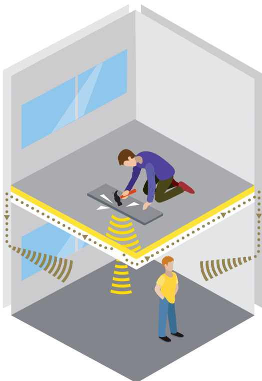
Recommended action Direct treatment of floor insulation
